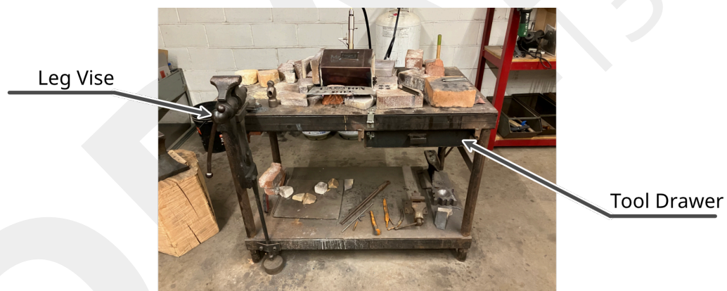
Figure 5: An annotated view of the large forge table.
