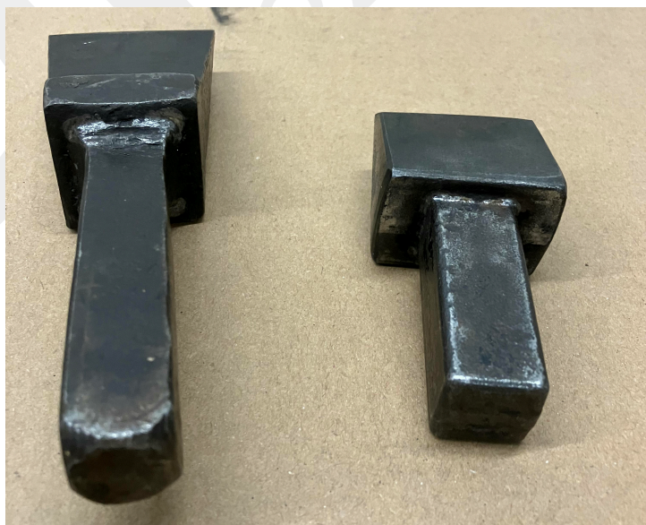
Figure 11: Two cutting tools. Note the square profile of the stems.
