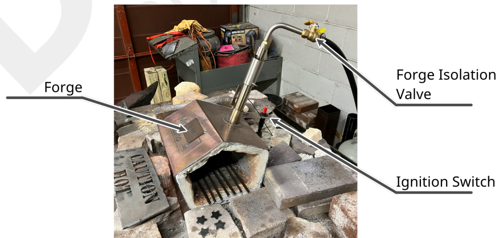
Figure 2: An annotated view of the parts of the forge.
