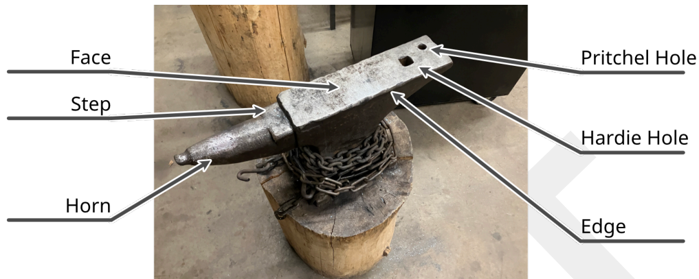
Figure 3: An annotated view of the parts of the anvil.
